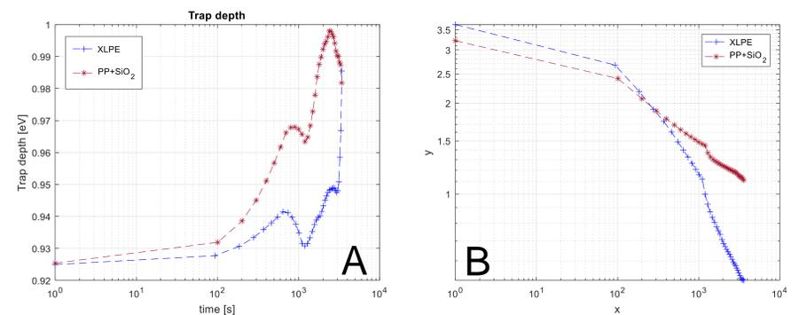
Fig. 4. Trap depth distribution in XLPE and cable-grade nanofilled polypropylene (A, after [2]) and their depolarization characteristics (B).
