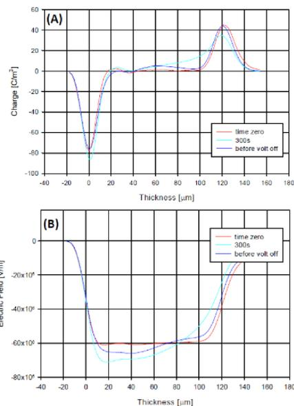
Fig. 2. Space charge (A) and electric field profile (B) measured at the beginning, during and at the end of polarization with (laplacian) field of 60 kV/mm. The maximum field bulk material is subject to is about 70 kV/mm, after 300 s.
