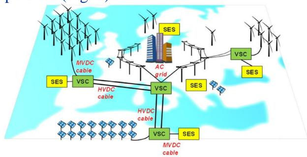
Fig. 1. Fields of application of the GRIDABLE project. SES stands for Stationary Energy Storage and VSC is Voltage Source Converter
