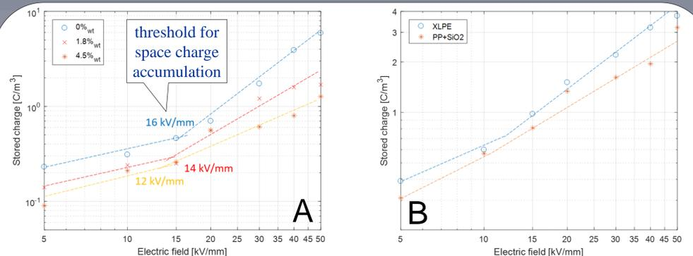
Fig. 3. Space charge characteristics for PP pure and filled 1.8 wt% and 4.5 wt% (A) and performance comparison with XLPE (B).
