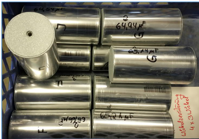
capacitor elements used for step-test
