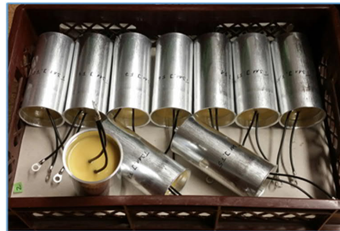
single element capacitors used for endurance test
